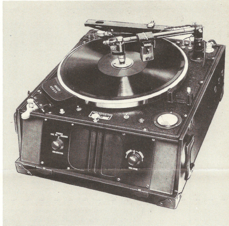
Presto Model "X" Recorder, similar to the Model "E", except that it is equipped with a 16" turntable. Makes and plays records up to 17 1/4" size at either 78 or 33 1/3 R.P.M. and operates as a public address system. Price, including Velocity or Crystal Microphone, Adjustable Floor Stand and Presto High Fidelity Cutting Head (range 50 to 7,000 cycles), $560.00.
