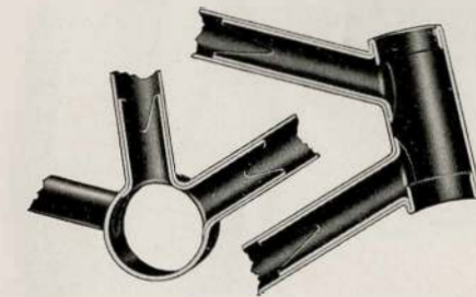
Cut open frame joints show the reinforced joint construction
