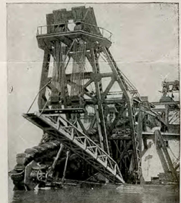
FIG. 7. PLACER DREDGE USED FOR HYDRAULIC MINING OF GOLD, TIN, Etc. Manganese Steel Buckets
