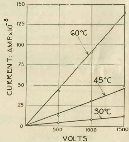
FIG. 17—VARIATION OF INITIAL CONSTANT CURRENT WITH VOLTAGE. OIL SPECIMEN B7.
