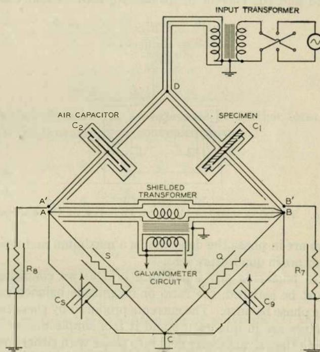
FIG. 1—GALVANOMETER CIRCUIT—DIAGRAM OF CONNECTIONS
