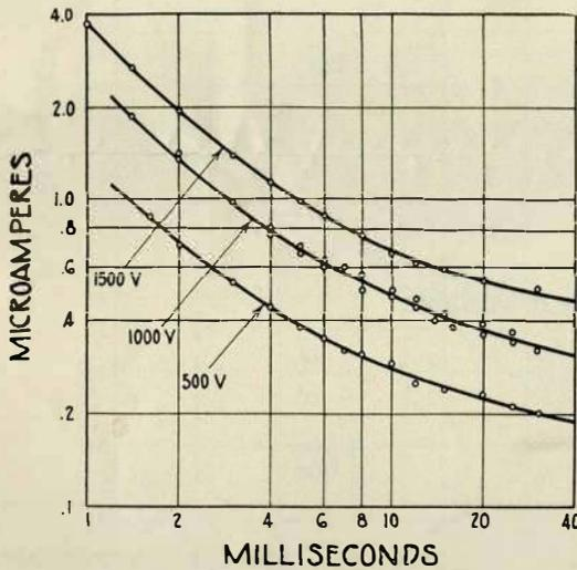
FIG. 3-VARIATION WITH VOLTAGE OF DISCHARGE CURRENT TIME RELATIONS AT 60°C. IMPREGNATED PAPER SPECIMEN C7. ILLUSTRATES DEPARTURE FROM  $t^{-n}$  EXPRESSION.
