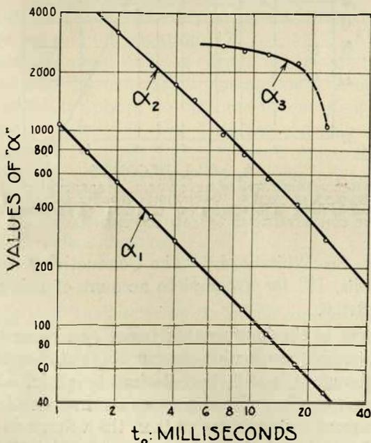
FIG. 7—VARIATION WITH  $t_0$  OF THE INVERSE TIME CONSTANT " $\alpha$ " OF EACH EXPONENTIAL
