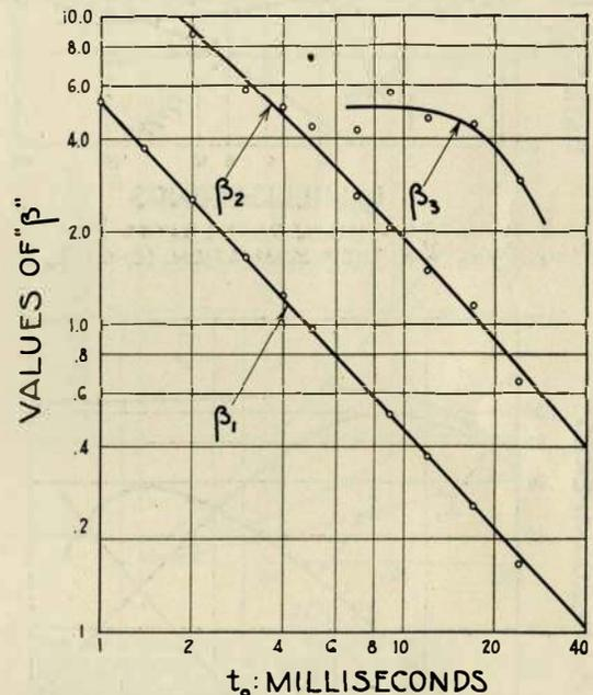
FIG. 8—VARIATION WITH  $t_0$  OF THE CONSTANT MULTIPLIER " $\beta$ " OF EACH EXPONENTIAL
