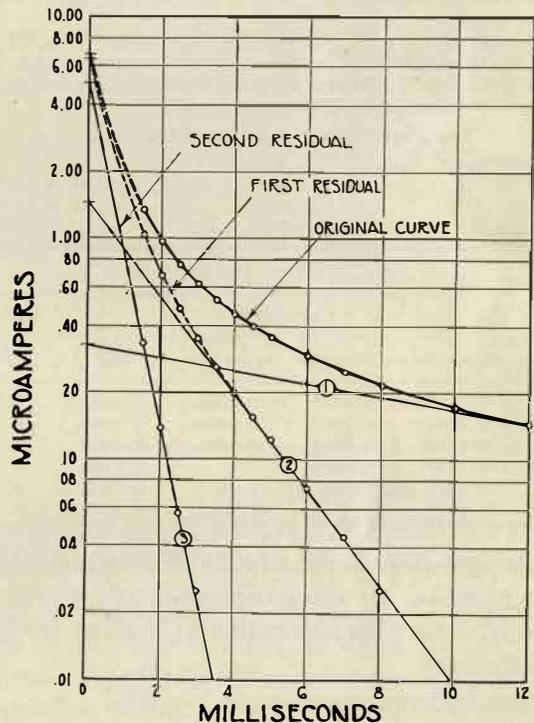
FIG. 4-APPLICATION OF THE METHOD OF THREE EXPONENTIALS TO A CHARGE AND DISCHARGE CURRENT-TIME RELATION AT 1500 VOLTS. DRY PAPER SPECIMEN A7 AT 60°C
