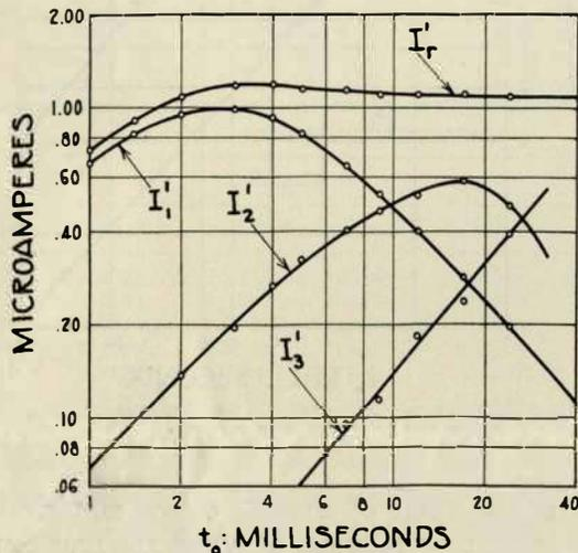
FIG. 10—CONTRIBUTION OF REVERSIBLE ABSORPTION AT 1500 VOLTS, 60 CYCLES. VARIATION WITH " $t_0$ " OF THE IN PHASE COMPONENT OF CURRENT ( $I'_r$ ) SHOWING THE CONTRIBUTIONS OF EACH EXPONENTIAL.
