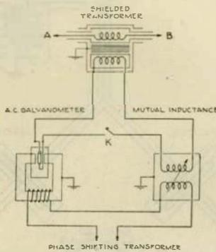
FIG. 2—GALVANOMETER CIRCUIT—DIAGRAM OF CONNECTIONS
