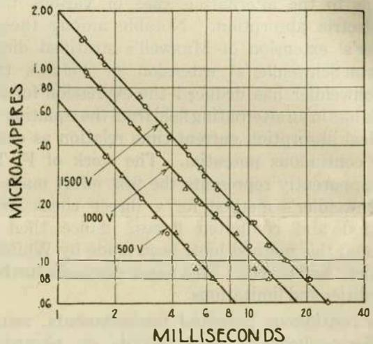
FIG. 2—VARIATION WITH VOLTAGE OF CHARGE AND DISCHARGE CURRENT-TIME RELATIONS AT 60°C. DRY PAPER SPECIMEN A7. ILLUSTRATES AGREEMENT WITH  $t^{-n}$  EXPRESSION FOR VALUES OF  $n > 1$ .
