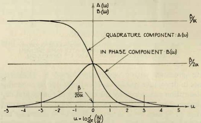
FIG 5—VARIATION WITH FREQUENCY OF THE IN PHASE AND QUADRATURE COMPONENTS OF A SINGLE EXPONENTIAL.
