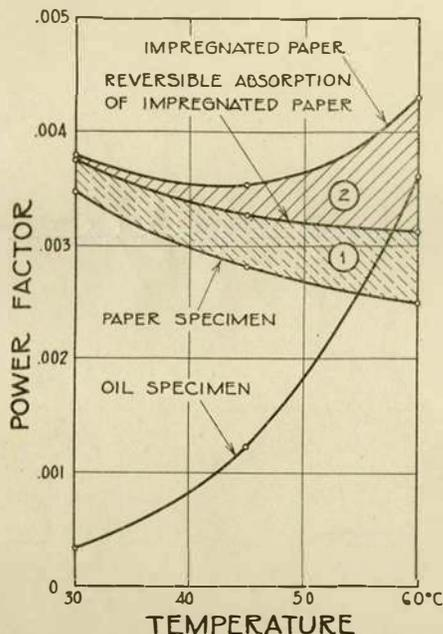
FIG. 21—ANALYSIS OF POWER FACTOR AT 1500 VOLTS. IMPREGNATED PAPER SPECIMEN C7
