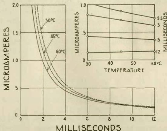
FIG. 15—VARIATION WITH TEMPERATURE OF CHARGE AND DISCHARGE CURRENT-TIME RELATIONS AT 1500 VOLTS DRY PAPER SPECIMEN A7
