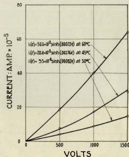
FIG. 12—VARIATION WITH TEMPERATURE OF CURRENT-VOLTAGE RELATIONS FOR THE INITIAL, CONSTANT, IRREVERSIBLE CONDUCTION CURRENT IMPREGNATED PAPER SPECIMEN C7.
