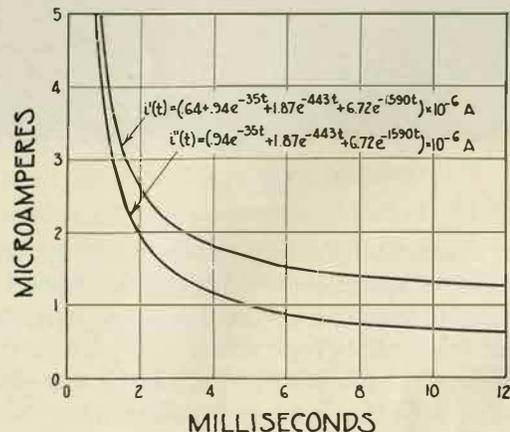
FIG. 20—CHARGE  $i'(t)$  AND DISCHARGE  $i''(t)$  CURRENT-TIME RELATIONS AT 1500 VOLTS, 60°C. IMPREGNATED PAPER SPECIMEN C7.
