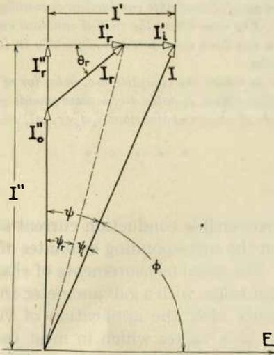
FIG. 1—VECTOR DIAGRAM OF A CAPACITOR SHOWING REVERSIBLE ABSORPTION AND IRREVERSIBLE CONDUCTION IN ADDITION TO SPECIFIC INDUCTIVE CAPACITY
