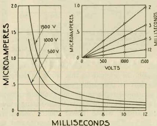
FIG. 14—VARIATION WITH VOLTAGE OF CHARGE AND DISCHARGE CURRENT-TIME RELATIONS AT 60°C DRY PAPER SPECIMEN A7.
