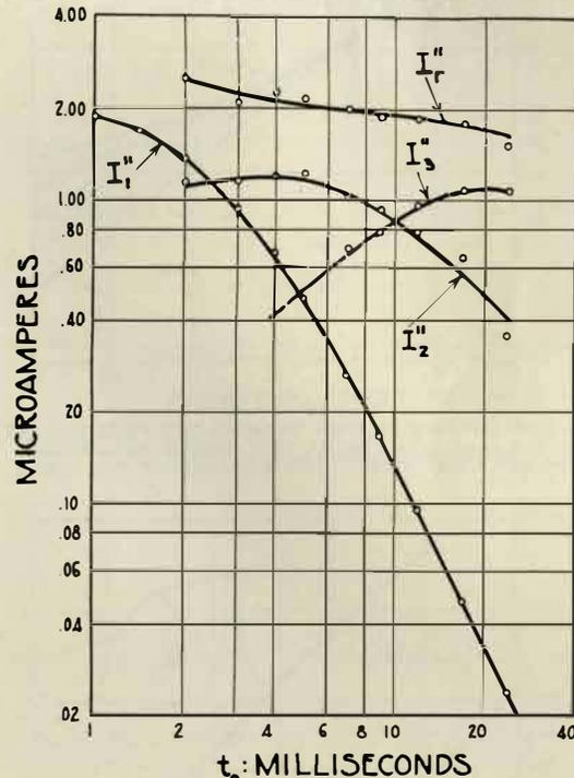
FIG. 11—CONTRIBUTION OF REVERSIBLE ABSORPTION AT 1500 VOLTS, 60 CYCLES. VARIATION WITH " $t_0$ " OF THE QUADRATURE COMPONENT OF CURRENT ( $I''_r$ ) SHOWING THE CONTRIBUTIONS OF EACH EXPONENTIAL.
