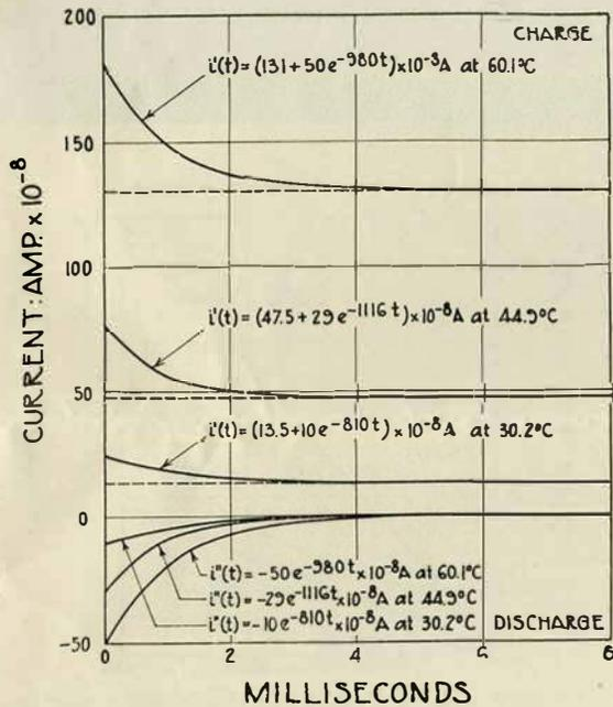
FIG. 18—VARIATION WITH TEMPERATURE OF CHARGE AND DISCHARGE CURRENT-TIME RELATIONS AT 1500 VOLTS. OIL SPECIMEN B7
