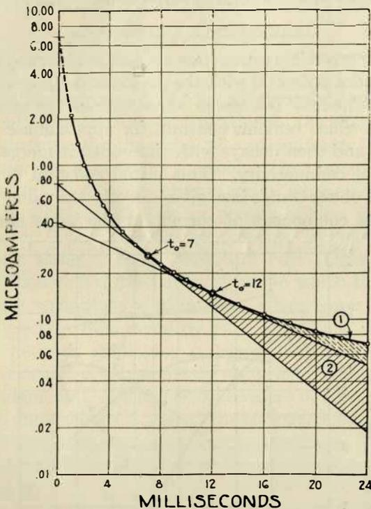
FIG. 6—CURRENT-TIME RELATION SHOWING THE FIRST TANGENT DRAWN AT TWO DIFFERENT VALUES OF  $t_0$ . SHADED AREAS SEGREGATE IN EACH CASE THE NEGLECTED PORTION OF THE CURVE
