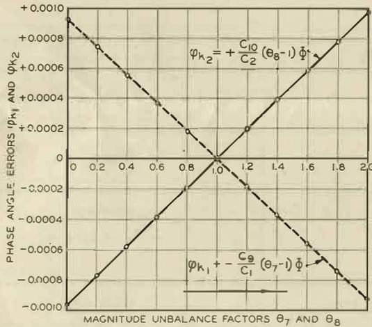
FIG. 4—EXPERIMENTAL VERIFICATION OF CASE 2
